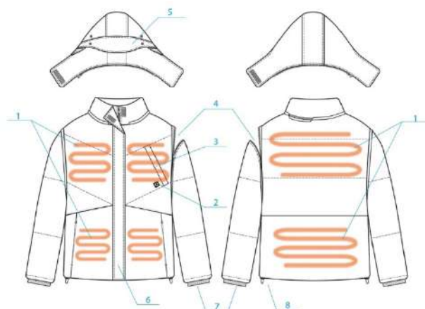
Fig. 10. Technical drawing of an improved heated jacket with the designation of the main places of design features
